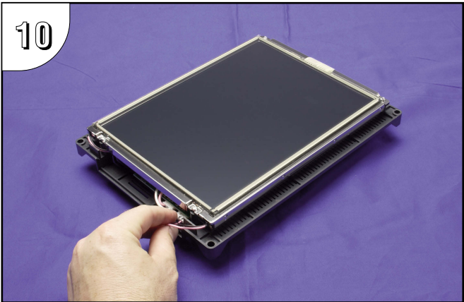
10 Plug each backlight bulb's power cable connector back into its respective circuit board connector.
