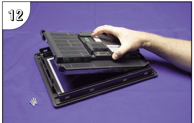
Position the touch panel's main electronics housing into the front bezel so that the flat ribbon cable on the housing aligns with the recess in the front bezel. Insert the four screws and tighten to a maximum of 70 oz-in [0.5 Nm].
