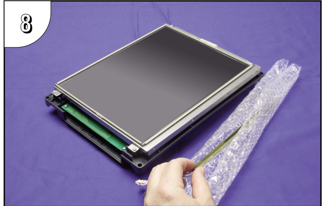
Remove the replacement bulb from its shipping tube and the protective bubble wrap.
