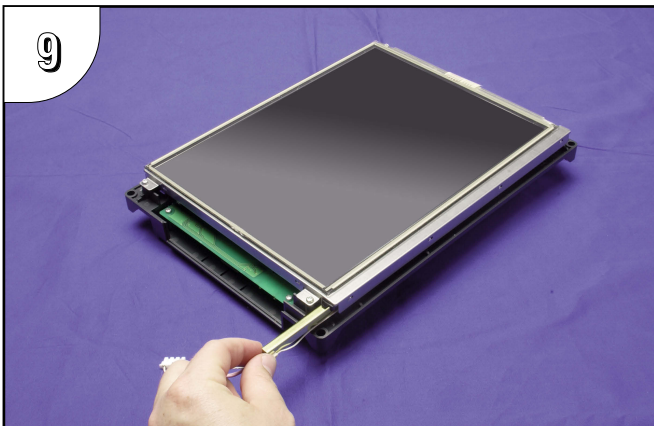
Position the replacement bulb so that the opening in its three-sided gold colored reflector faces toward the LCD touch screen. Using gentle pressure, slide the bulb into the guide until the retaining clip locks.
