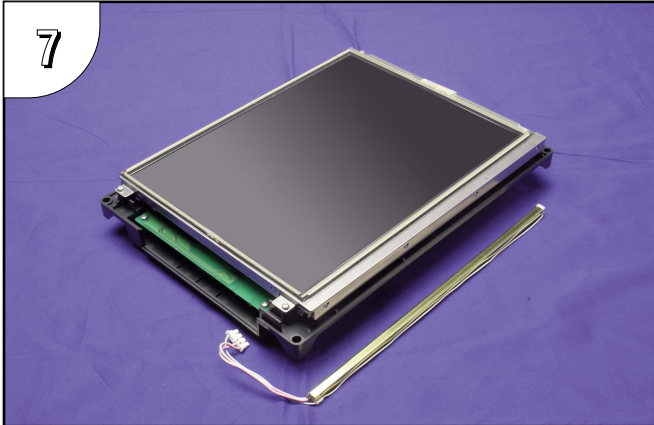
This photo shows the backlight bulb completely removed from its guide in the panel's main electronics housing.
