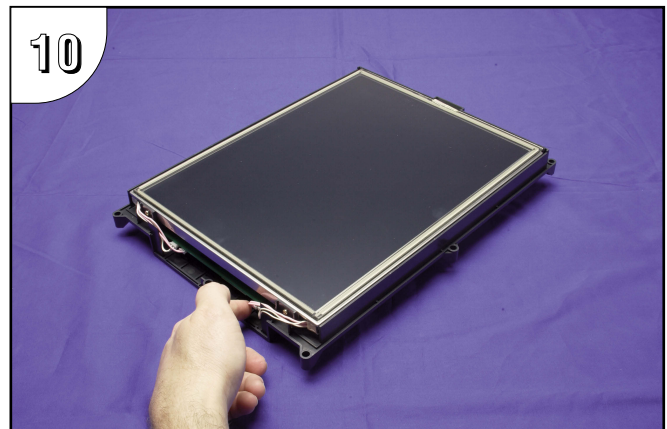
10 Plug each backlight bulb's two power cable connectors back into their respective circuit board connectors. Each bulb's two connectors are keyed to prevent mismatching.
