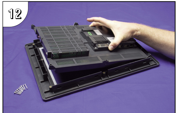
12 Position the touch panel's main electronics housing into the front bezel so that the flat ribbon cable on the housing aligns with the recess in the front bezel. Insert the eight screws and tighten to a maximum of 70 oz-in [0.5 Nm].
