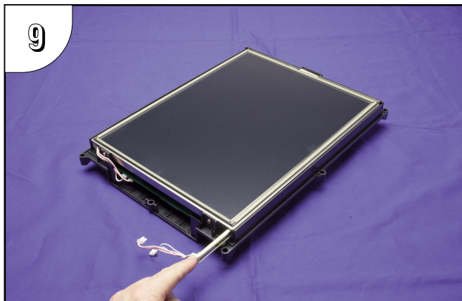
9 Position the replacement bulb so that the opening in its three-sided gold colored reflector faces toward the LCD touch screen. Using gentle pressure, slide the bulb into the guide until it is flush with end of guide.
