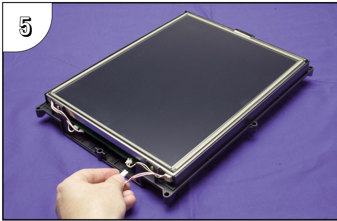
5 Unplug each backlight bulb's two power cable connectors from the circuit board connectors. Again, do this for both the upper and lower backlight bulbs.
